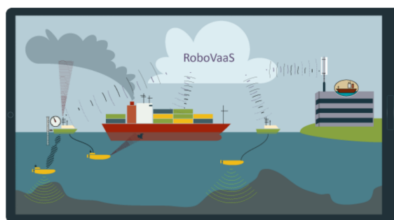
Figure 1: RoboVaaS envisioned example scenario showing ship-hull inspection and anti-grounding services enabled through a fleet of ROVs and UUVs connected with acoustic underwater and radio communication.
