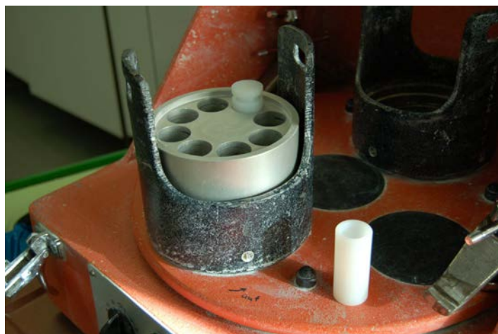
Fig. 4.3 High-throughput compatible planetary mill. The bigger milling containers were modified to accommodate 16 smaller milling containers to facilitate simultaneous milling. The smaller milling containers were made from ultra-high-molecular-weight polyethylene (UHMPE).
