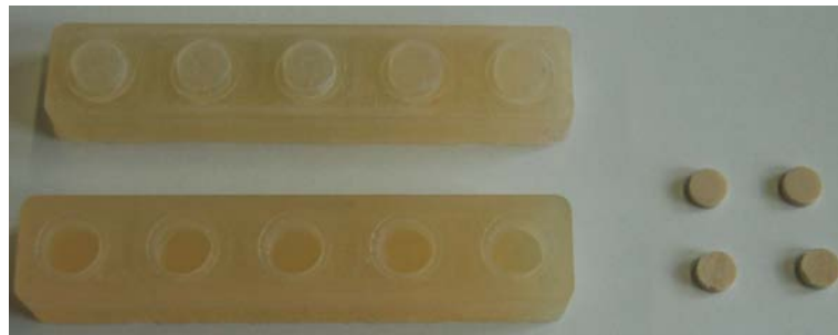
Fig. 4.5 Silicon mould adapted for use in cold isostatic press for both conventional and high-throughput synthesized powders.
