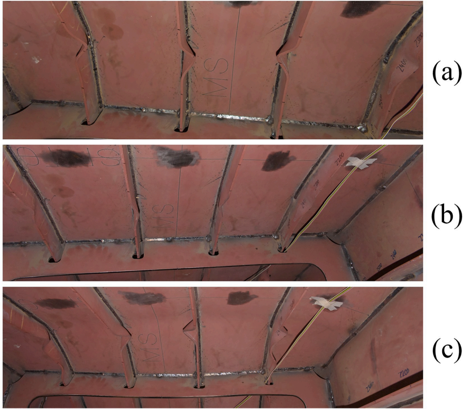
Fig. 17. Deformation of the stiffeners on top hull in S2, (a) - (c) refer to the results after 1st, 2nd and 3rd half-cycle respectively. In the picture, the right side is closer to starboard.
