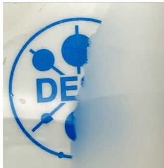
Figure B.1: Mesoporous glass that is transparent where saturated with water or opaque in a region partially dry blown.
