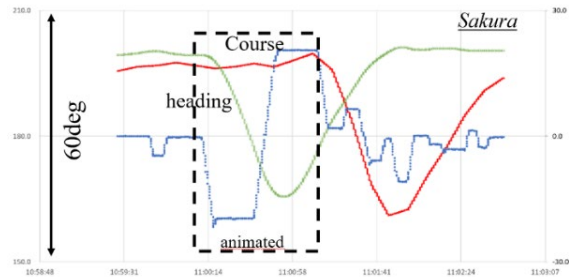
Figure 3: Relationship between the heading angle and the ship course for Sakura
