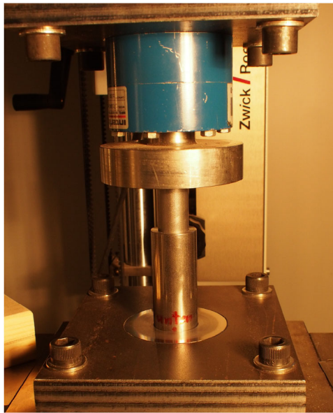
FIGURE 3 Experimental setup for multi-particle compression tests.
