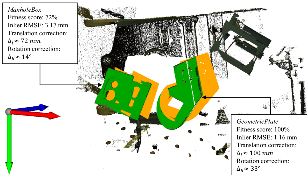
Figure 8. Refined pose achieved using ICP. The coordinate frame represents the origin of the target point cloud. Meshes in orange show the estimated 6D pose, and meshes in green show the improved results.
