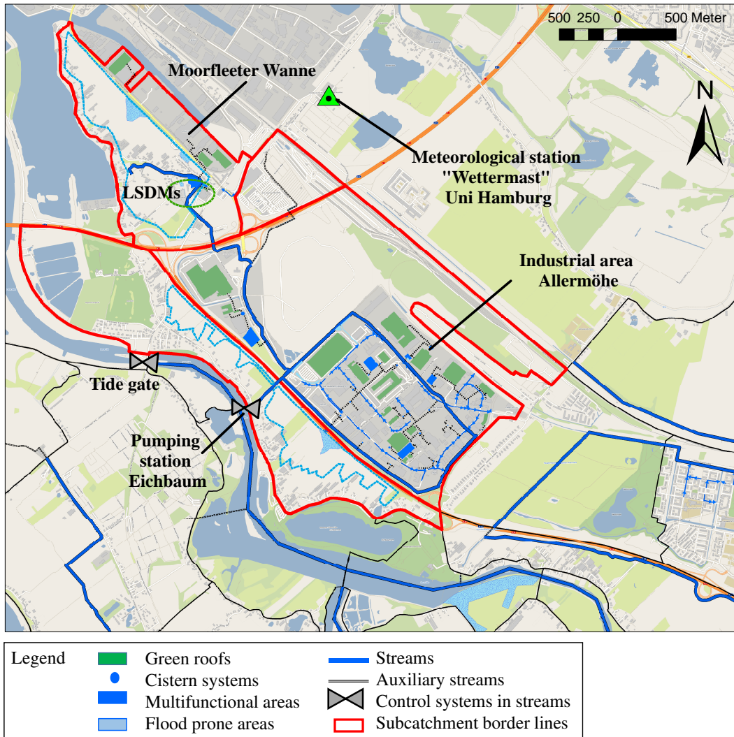
Figure D.33: Map of LSDMs installed in the Moorfleet study areas [Scenario 3] (background map: www.ows.terrestris.de ).
