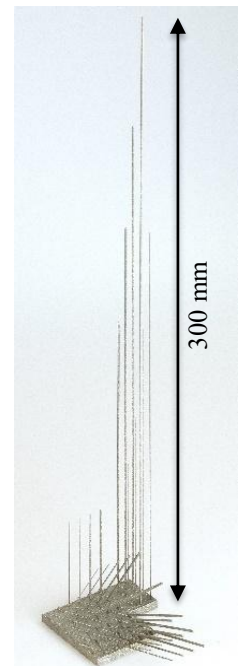
Figure 1: Parameter study on thin rods manufactured by AM. The scale is given by the tallest rod with a height of 300 mm.
