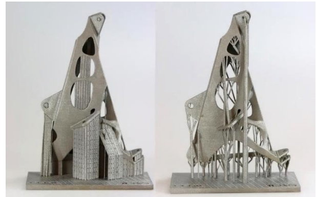
Figure 4: Additively manufactured demonstrator part with block supports (l.) and tree supports (r.)
