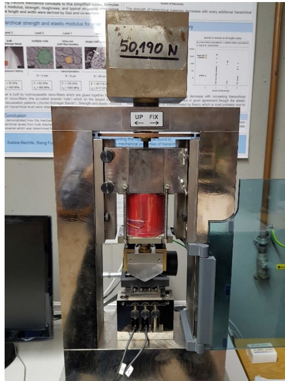
Figure 31: Mechanical arrangement for the force calibration.
