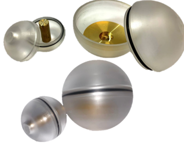
Figure 2.11: LSPs with 25 mm equatorial LP and cylindrical brass insert (top left). The 40 mm off-centre LP with a brass insert with unbalanced mass distribution (top right). Closed 25 mm equatorial and 40 mm off-centre LP (bottom)[Rau23]
