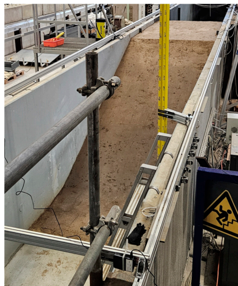
Figure 1. Dike construction within the experimental concrete channel at RWTH Aachen.
