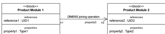
Fig. 3 BDD of a product module associated with another product module via its assembly requirement formulated as a DIN8593 joining operation
