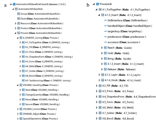
Fig. 5 (a) Process RCL with joining processes, handling and additional functions. (b) Process SUCL with joining processes detailed by subfunctions
