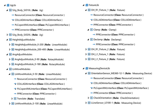
Fig. 11 SystemUnitClassLibraries of the available jigs, fixtures, and measuring devices for the configuration of a modular jig
