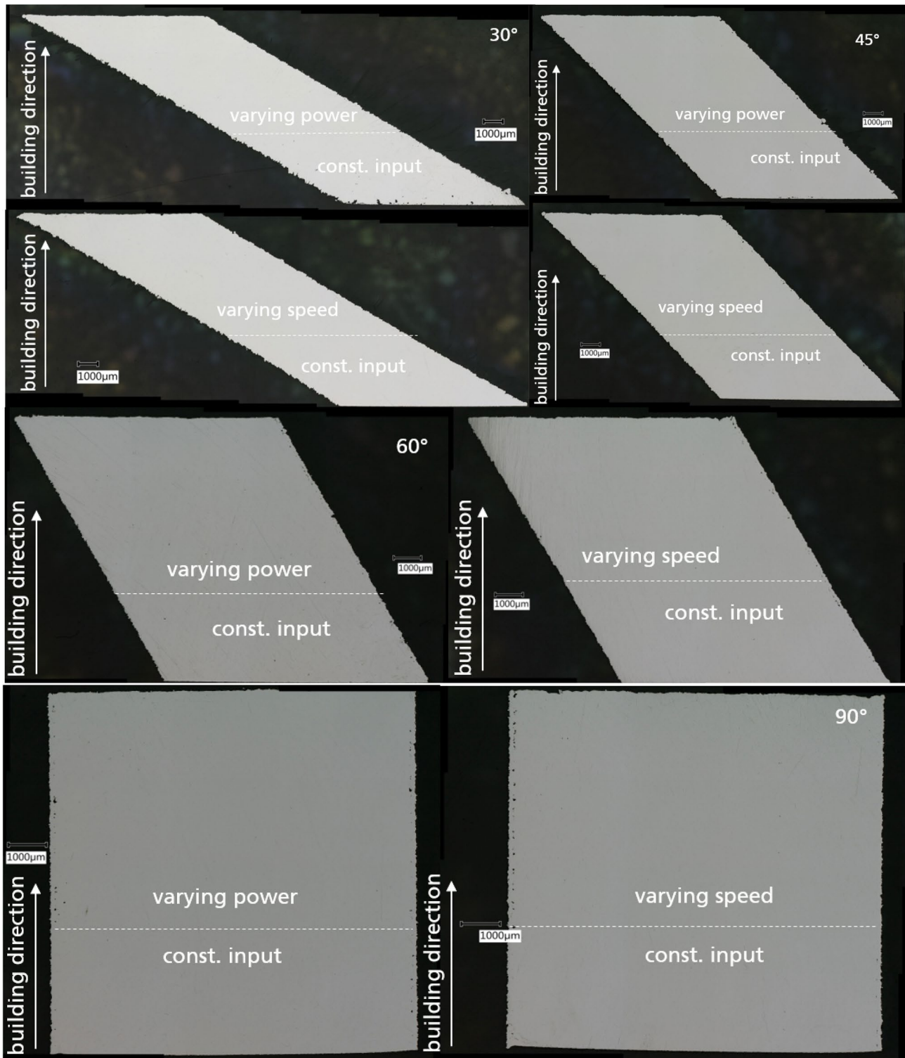
Fig. 14 Microscope image of the cross-section parallel to the building direction z -axis of 30, 45°, 60° and 90° specimens manufactured with both decreasing laser power and increasing scan speed over the height
