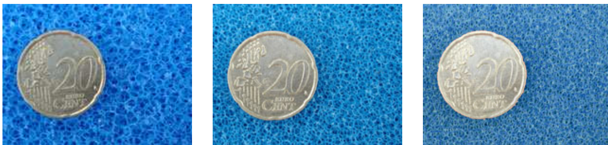
Figure 5.86: PU foams with different densities (10-30 ppi), taken from Saarschaum Saarbrücken, Germany - www.saarschaum.de
