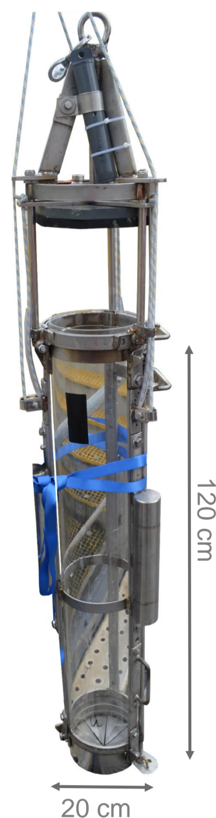
Fig. 1 Sediment core sampler developed by TUHH, IRCE (2019)
