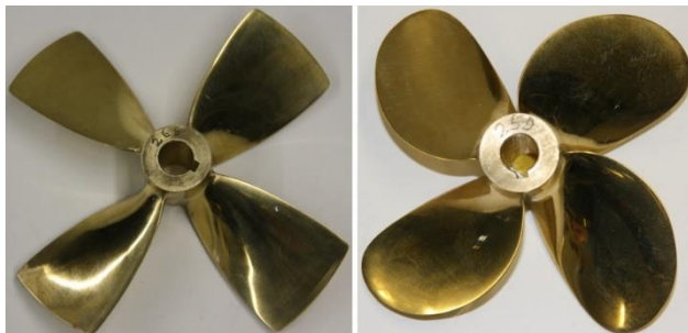
Figure 2. Right-handed propellers used in the experiments; Left: Kaplan P274r propeller; Right: Wageningen B4-70 propeller. Both propeller have a propeller diameter of D_p = 0.11 m and an hub diameter of D_h = 0.02 m.
