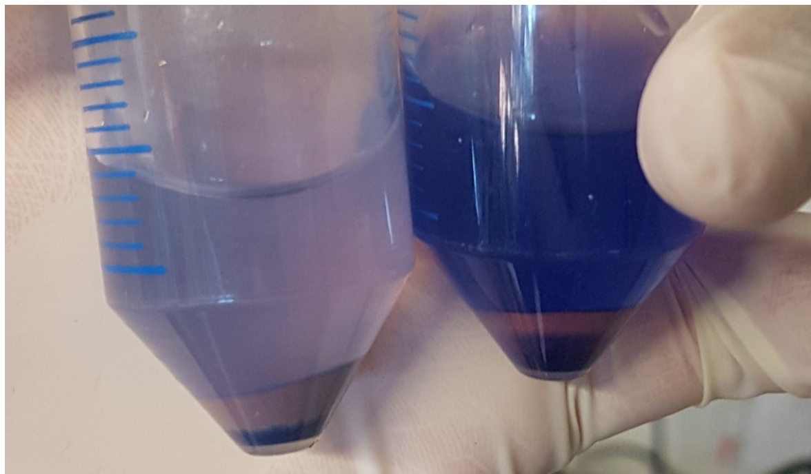
Figure 27: Supernatant of 10 mL R. toruloides culture broth (82 h of process time) after centrifugation at 7000 g for 10 min. Left: Addition of 60 mg L -1 Brilliant Blue and application of -0.4 A at pO 2 = 5% (Microaerobic BB CEF). Right: Addition of 60 mg L -1 Brilliant blue at pO 2 = 5% without application of electricity. Picture taken by the author.
