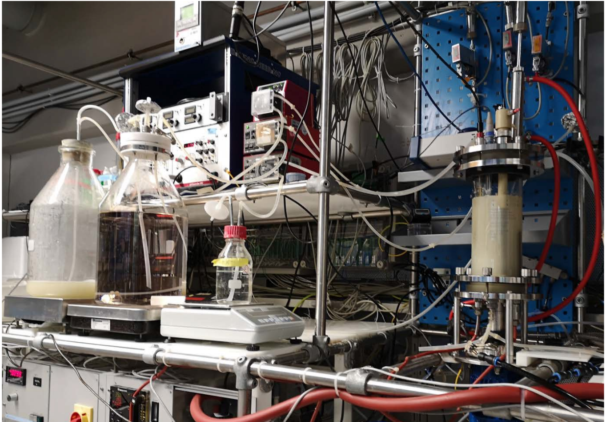
Figure 17: Experimental set-up for the electricity-aided continuous cultivation of C. pasteurianum in a system with automated fast-filtration.
