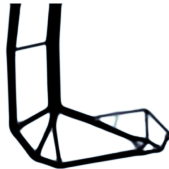
Figure A.4: Obtained density distribution and convergence plots of volume-constrained optimizations. Aggregation is performed by means of the p -norm function.
