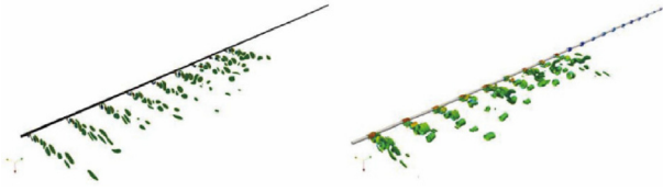
Fig. 3. Vortex shedding of a flexible riser predicted by 2D and 3D strip theory. Reproduced from Ref. [68] with permission of Elsevier, ©2020.
