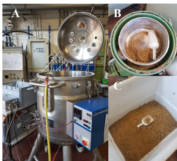
Figure 6.5: Images of A) 400 L bioreactor setup, B) solid-liquid separation by centrifugal forces (separator), and C) P-reduced rye bran.
