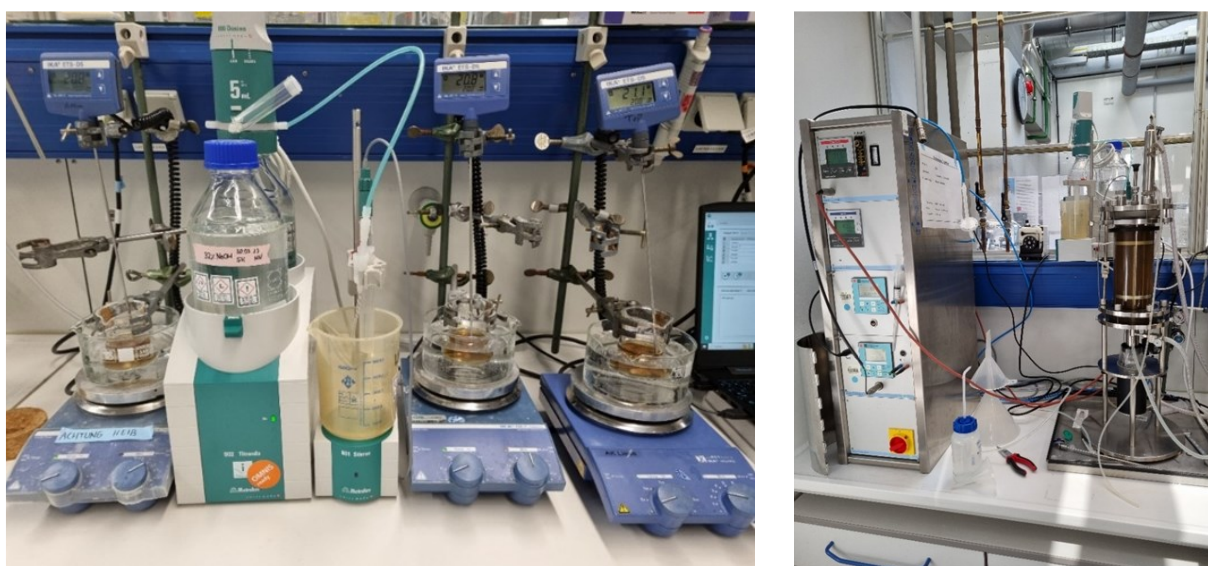
Figure A.2.6: Left : Experimental setup for struvite precipitation in glass beaker, and right : during scaling of the precipitation (right).
