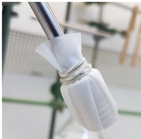
Figure 4.17: Original image of the optical fibre enclosed by the membrane module.
