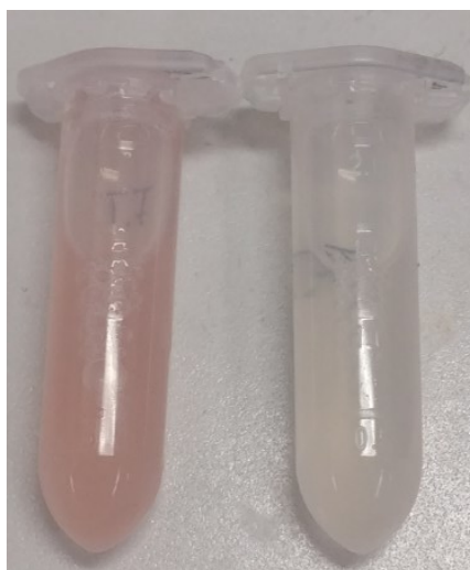
Figure B.1: Coloring of the bran extract by anthocyanins. The eluent of the ion exchange chromatography is shown. Loading of the IEX column with 5 mL bran extract diluted 1 to 5. Elution with 4 mL HCL. Left : Washing step with 8 mL 0.05 M HCL and right : subsequent elution with 4 mL 2 M HCL.
