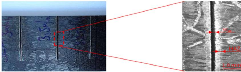
Fig. 2. Cutting kerfs and extension of HAZ
