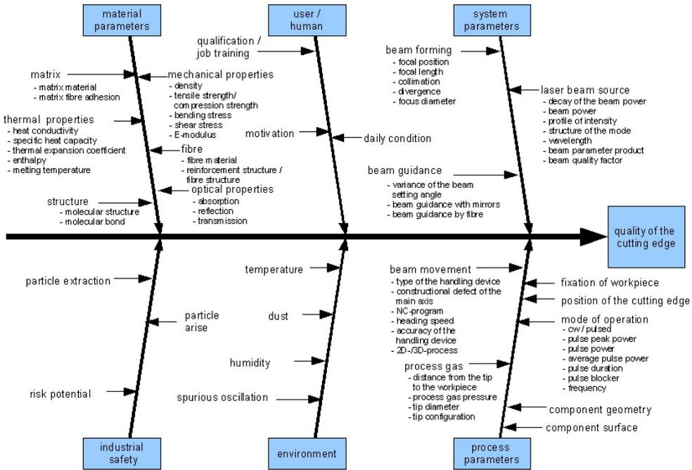
Fig. 3. Cause-Effect-Diagram of laser beam cutting of CFRP
