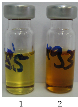
Figure 2.27: Colour change of the permeate due to catalyst injection, (1) c_{catalyst,1} = 35 \text{ mmol L}^{-1} end of period B and (2) c_{catalyst,1} = 70 \text{ mmol L}^{-1} after catalyst injection beginning of period C
