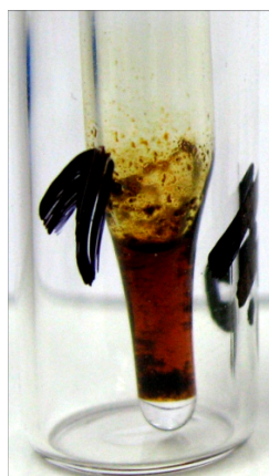
Figure 2.9: Adhered catalyst at the glass walls of the reaction vial after sampling
