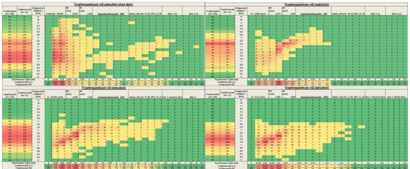
Figure 8. Example of output of rainfall character: drop size vs fall velocities
