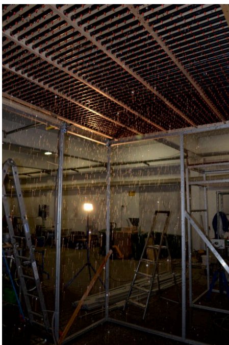
Figure 6. Rainfall demonstration without net, RS-TUHH
