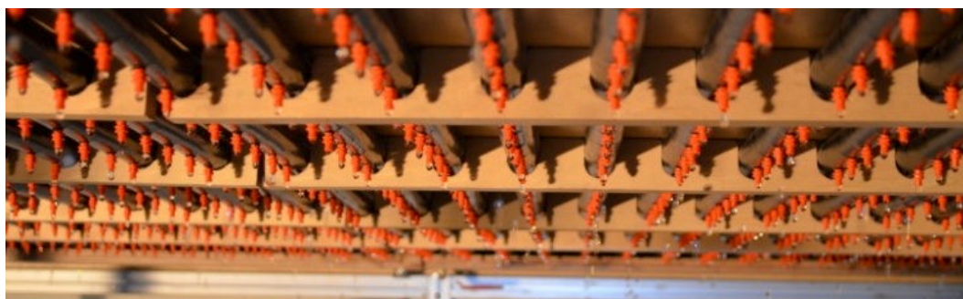
Figure 3. Single drop creation method “endline drip heads”
