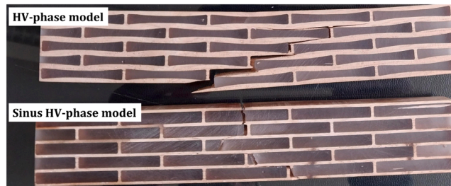
Fig. 10. crack growth morphology in the studied Sinus-HV phase and HV phase models' structure.
