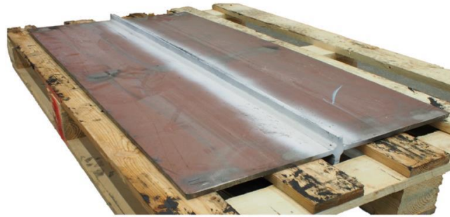
Figure 3.2: Welded plate before sawing [Brau20a]
