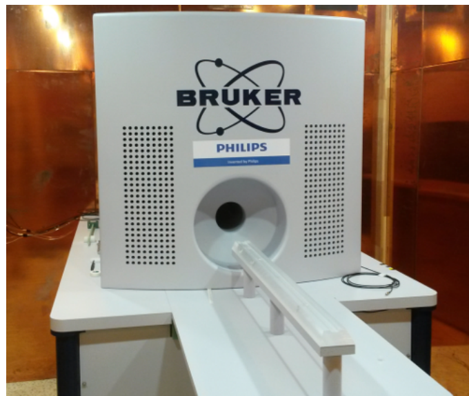
Figure 2.20.: Bruker scanner inside room with copper shielding.
