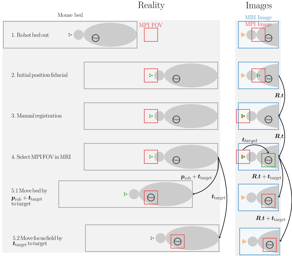
Figure 4.6.: The MRI-based selection of MPI FoV can be described in five steps. 1. Acquire MRI image, 2. Identify the fiducial in MPI, 3. Perform the registration, 4. Select target FoV, 5. Move to selected target FoV.
