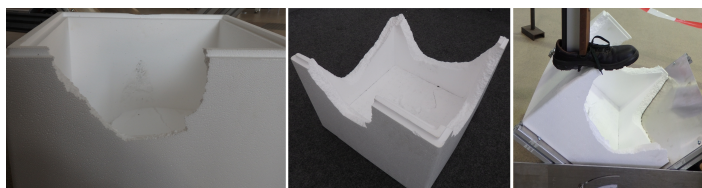
Figure 5: a. Rupture shape from the first side of the bigger box. b. Remaining of the box, once all the sides are broken. c. Procedure to break the remain-ing edges of the box.
