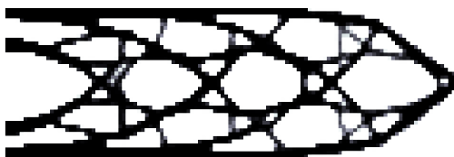
Figure 4.15 – Result for a fail safe cantilever beam from [37], obtained by TO using load-path-based damage directly.
