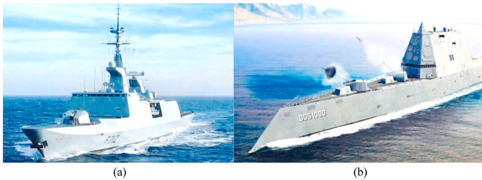
Fig. 14. Composite Superstructure on the ship (a) Lafayette frigate, (b) Zumwalt (DDG-1000) destroyer [45].
