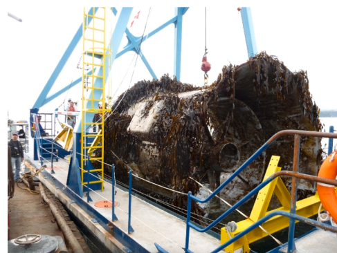
Fig. 12. Environmental degradation of composites for marine current turbine [41].
