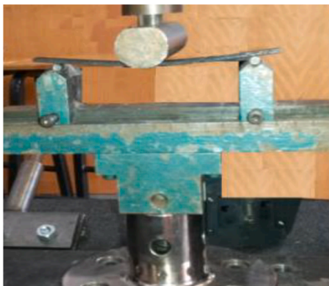
Fig. 37. Three-point bending test on the Instron 3367 machine [111].
