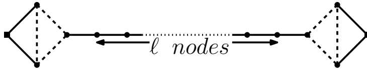
Figure 3.2: An instance on which the multi-depot subtour-elimination LP has integrality gap arbitrarily close to 2. The square vertices are the depots and all edges have unit weight. The dashed edges are assigned x_e = 0.5 by the LP, the other edges x_e = 1 . The LP then has optimum value at most \ell + 6 , whereas the MDMTSP has optimum value 2(\ell + 4) .
