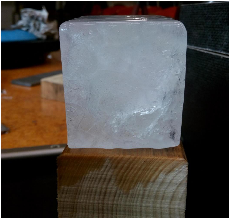
Figure 19: Crack can be seen through the surface of the cracked specimen
