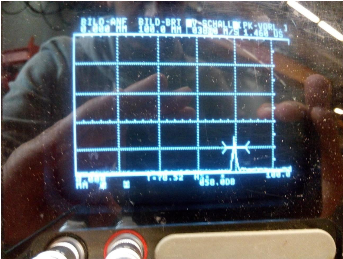
Figure 26: An indicated back wall echo at the length T = 78.52
