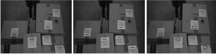
Figure 7: From left to right: Original camera image, detecting relevant barcodes (ignoring others) and decoded barcodes.
