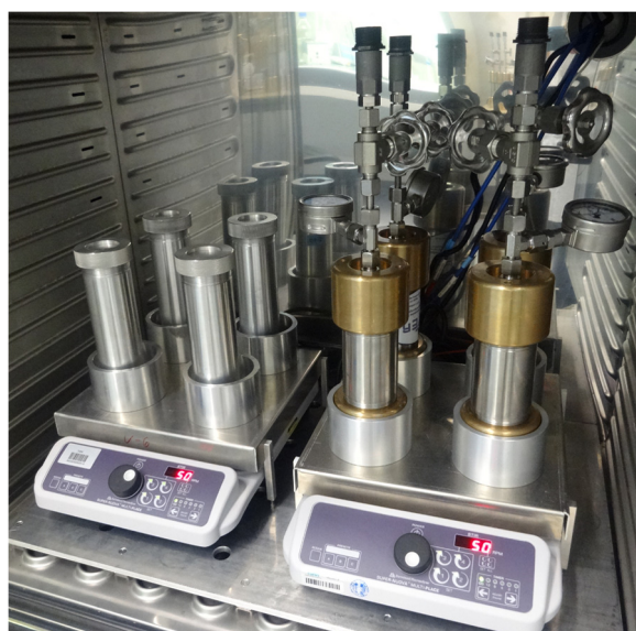
Figure 1 High-pressure reactors and control reactors. High-pressure reactors (right, made from stainless steel and bronze, max. pressure 40 MPa, pressurizing with N 2 gas, 160 mL volume) and aluminum control reactors (left, max. 0.1 MPa, 160 mL volume) were used for cultivation of hydrocarbon degraders at high and ambient pressure. The cultures were mixed with magnetic stirrers.
