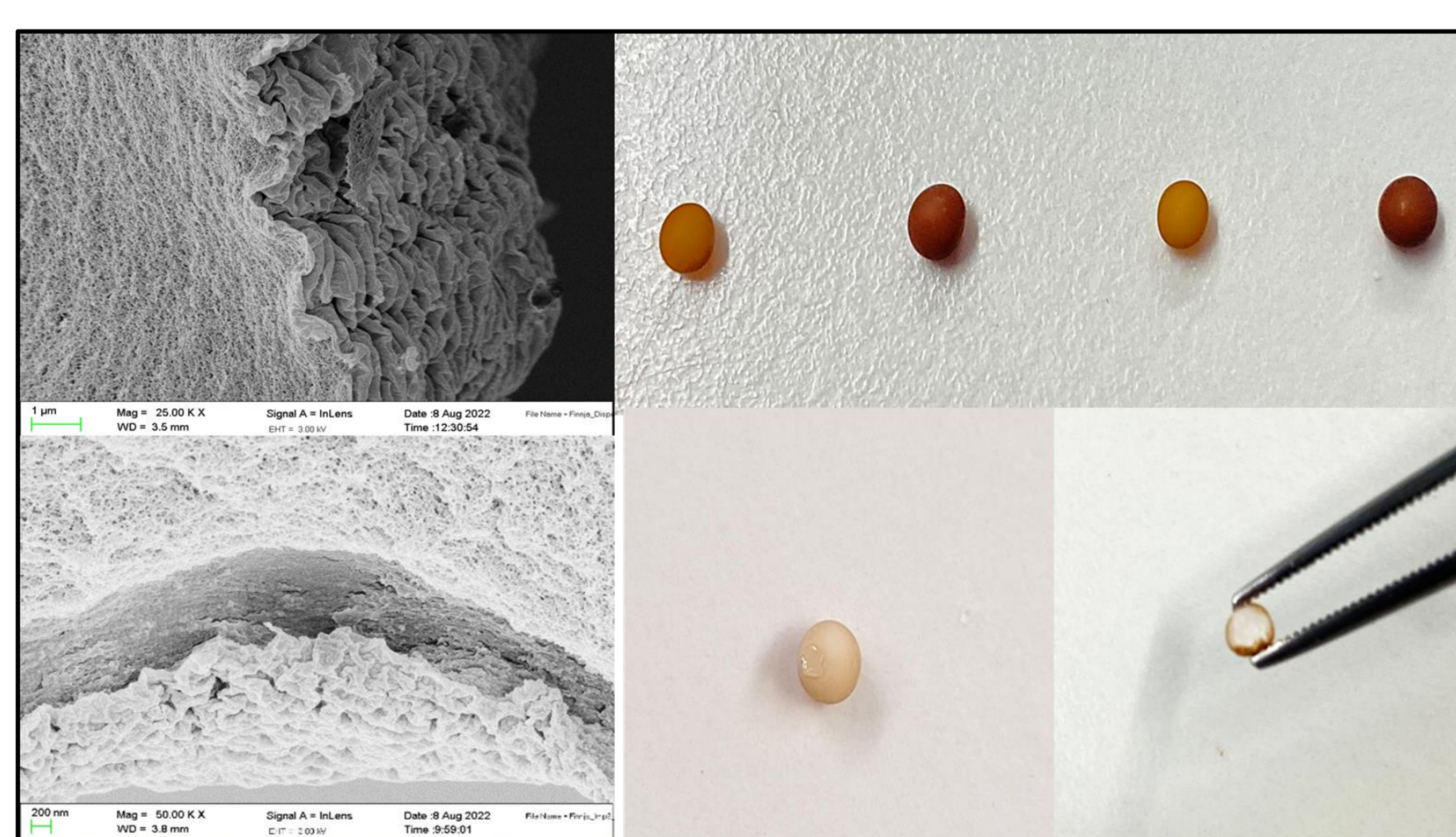
Fig.4 SEM image of the Lignin coated alginate shell-core aerogel particle.
