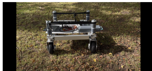
Figure 5. First telescopic lightweight modular robotic platform prototype.
