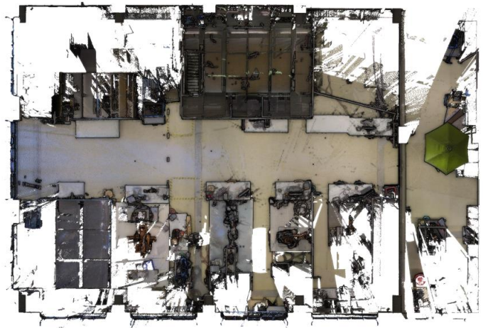
Figure 3: 3D scanned ground truth data of our research laboratory captured with a Leica BLK360G2.
