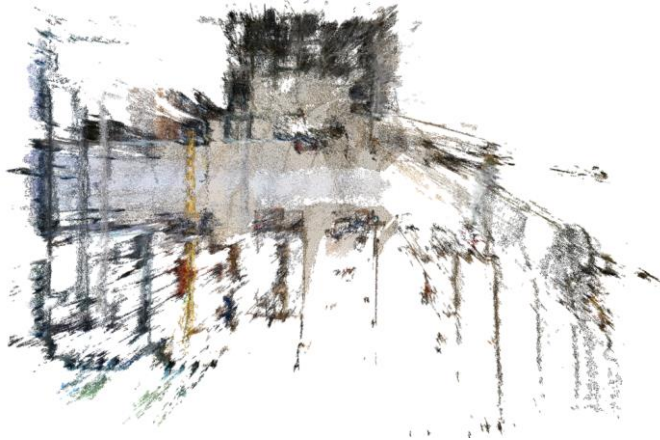
Figure 5: 3D reconstruction of the laboratory environment with our Structure-from-Motion (SfM) pipeline.
