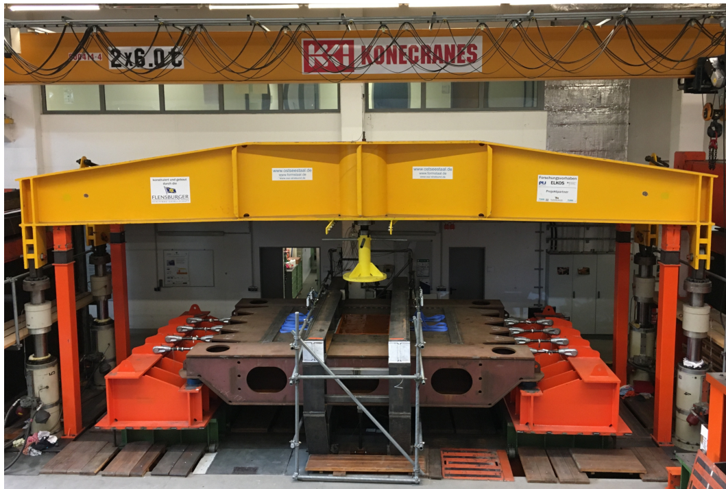
Figure 3.5.: Experimental set-up of the large-scale ice extrusion test for 800 mm specimens without confining pipe
