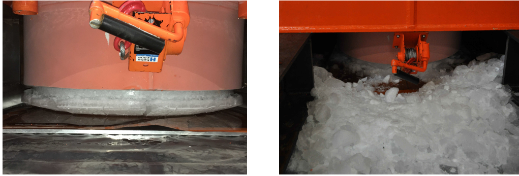
(a) Ductile test: Cone800_G100_A20_V01 (b) Brittle test: Cone800_G100_A20_V4_1
