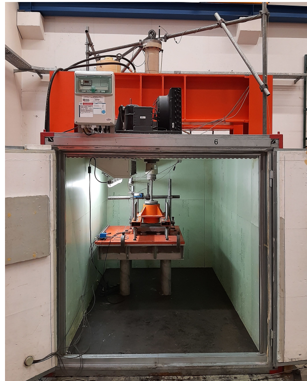
Figure 3.3.: The used test rig and cold room for the small-scale tests with 100 mm and 200 mm specimens. In contrast to the actual test set-up used, the picture shows a 160 kN cylinder. The 1.3 MN cylinder used during the tests can be seen dismounted to the left of the 160 kN cylinder
