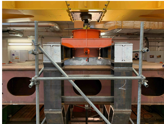
Figure 3.25.: Ice extrusion test Cone800_Panel2_G200_A20_V4 during testing
