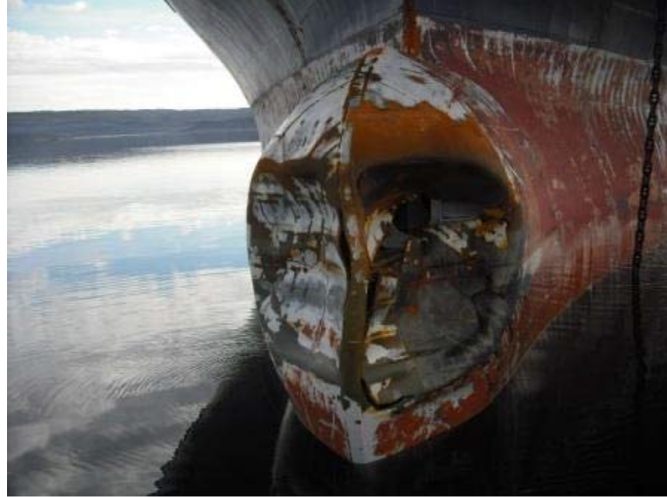
Figure 1.1.: Damaged bulbous bow of a cargo vessel with a Lloyd’s Register 100 A1 ice class after a collision with a Bergy Bit (Canadian Coast Guard, 2012)
