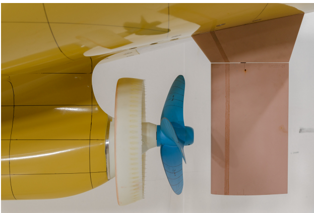
Figure 3: Prairie-like system developed for present model tests. Air is injected from needles mounted in the trailing edge of the duct upstream of the propeller rather than from holes in the propeller blade leading edges (as in the original Prairie system).
