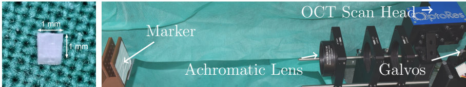
Figure 6.2: The experimental setup for data acquisition and annotation: Marker object (left); OCT setup (right). Figure adapted from [38].
