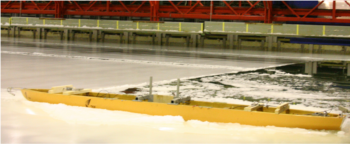
Fig. 2.2: Ship model at Aalto Ice Tank prior to a resistance test. The model ice contains 0.3 % of ethanol for the adjustment and scaling of strength. The ship is towed through an open channel, while the carriage is pushing the ice orthogonally to the moving direction of the ship applying a compressive frictional force onto the hull. Image: R. U. F. von Bock und Polach, with kind permission.
