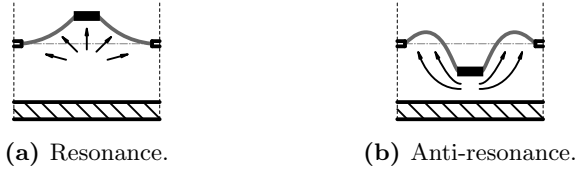
Figure 3.5: Qualitative displacement of a MAM in front of a wall at the first MAM resonance frequency and the first MAM anti-resonance frequency.
