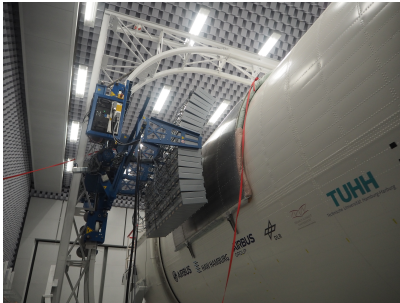
(a) Noise shield with loudspeaker array in position.
