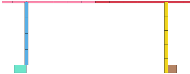
Fig. 20. The bulb flats in the numerical model of large structure, modelled with shell-only model (left half) and beam & shell model (right half). Shell thickness and beam prism are shown here.
