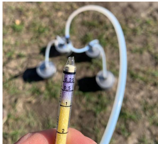
Figure 10 Indicator tubes as concentration measurement method for \text{NH}_3 in field trials (Dräger Tubes)
