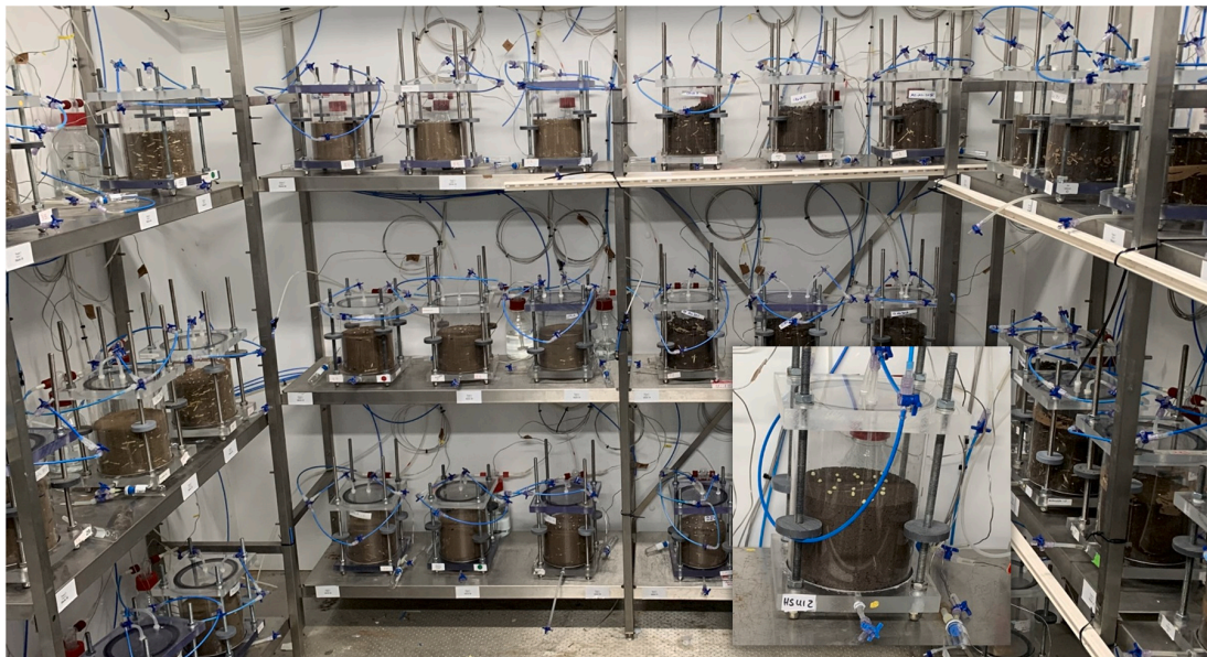
Fig. 1. Set-up of flow chambers for \text{N}_2\text{O} quantification.
