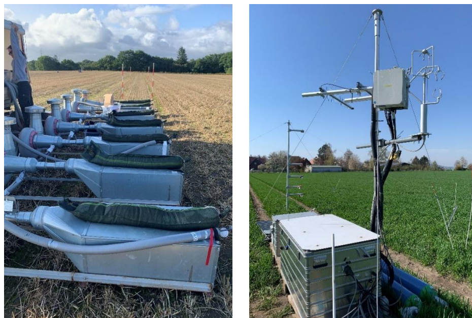
Figure 9 Concentration measurement methods for \text{NH}_3 in field trials left wind tunnels used with cavity ring-down spectroscopy and right quantum cascade laser
