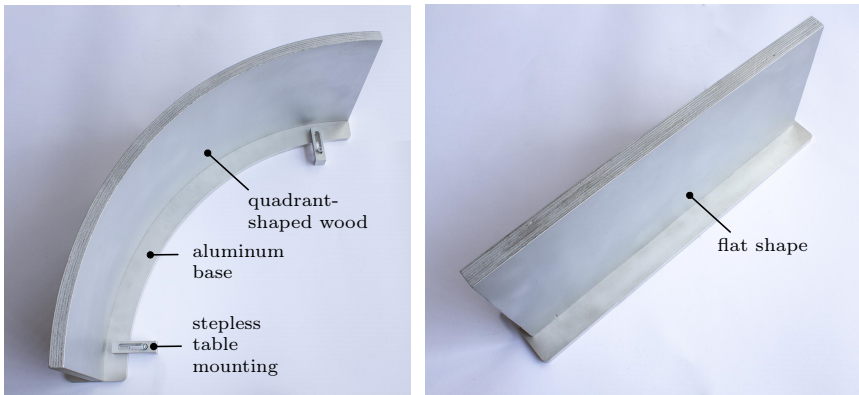
Figure 2.9: Circular and flat wood contact walls for force/motion control.
