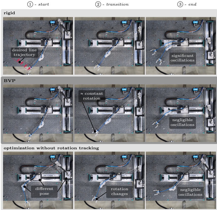
Figure 5.34: End-effector line trajectory tracking with constant rotation based on three different model inversion cases.
