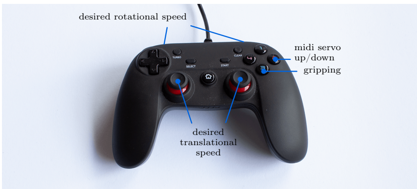
Figure 2.28: Utilized game pad with two vibration motors and XInput support.
