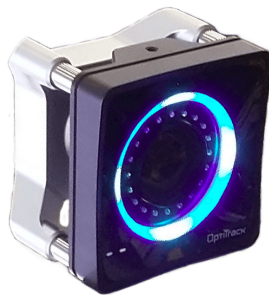
Figure 2.17: Motion tracking camera Prime 17W with active LED ring.
