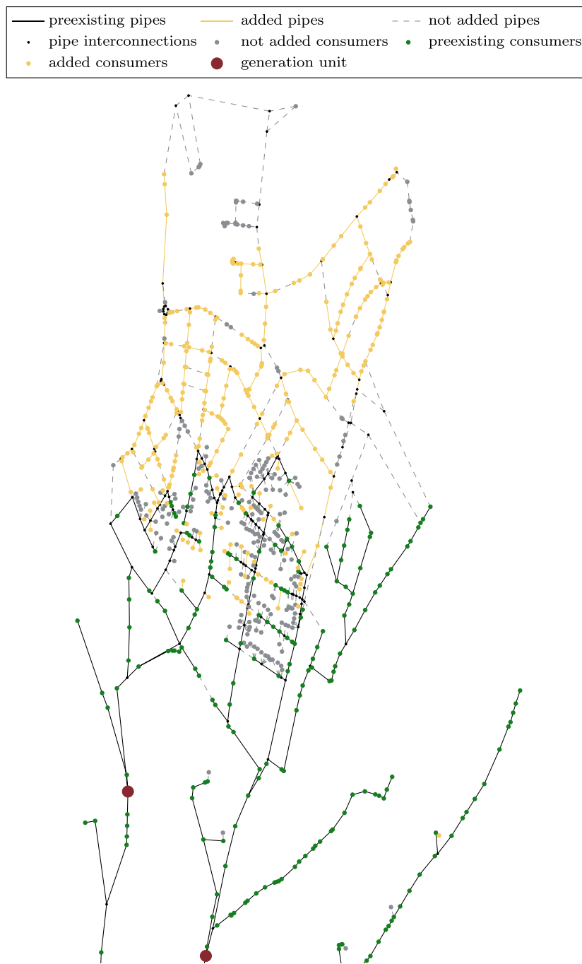
Fig. 6. Resilient expansion planning results with r = 0.05 \frac{\text{€}}{\text{kWh}} in the north eastern area with a high density of potentially new consumers.
