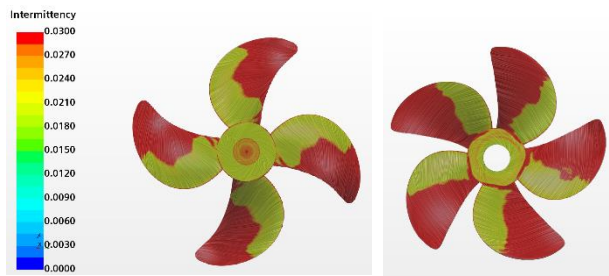
Figure 26 J=0.2 Laminar zones on FWD and AFT propeller as predicted by the transition turbulent
