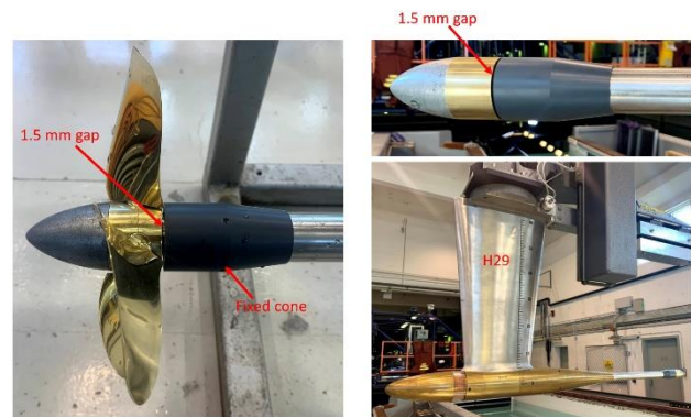
Figure 2 Set-up for open water tests
