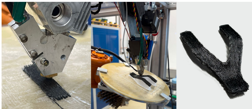
Fig. 12 Physical realization of the printhead during functional verification; part cooling vent and fan flipped up for better visibility. Left: printed coupon shows cuts, middle: non-planar printing with dynamic layer height variation, right: final printed part
