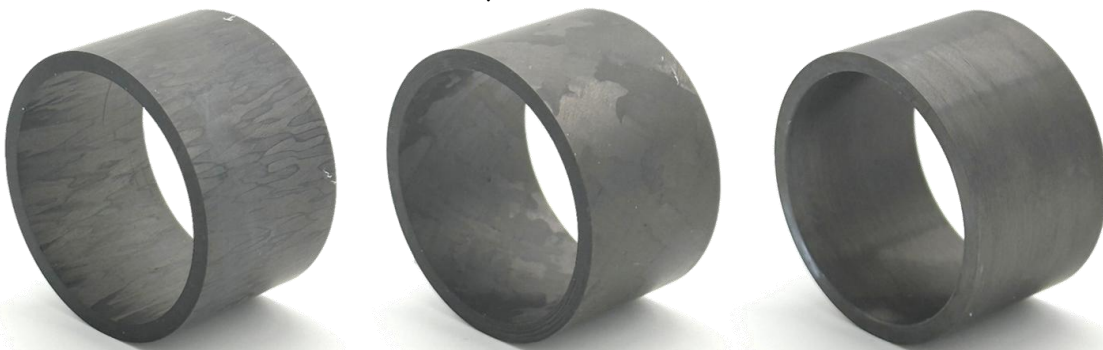
Figure 2: CFRP specimens in the orientations from left to right: winding angles of \pm 10^\circ , \pm 45^\circ , and \pm 89^\circ .
