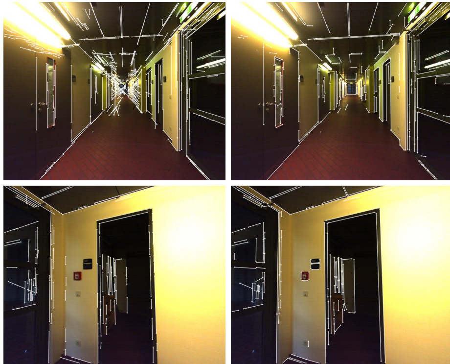
Figure 3.15: Comparison of the progressive probabilistic Hough transform (left) to Douglas-Peucker line segment detection with line fitting (right). For the tested scenes, computation times (30ms vs. 8ms on average) as well as detection quantity and quality are significantly superior in case of Douglas-Peucker.
