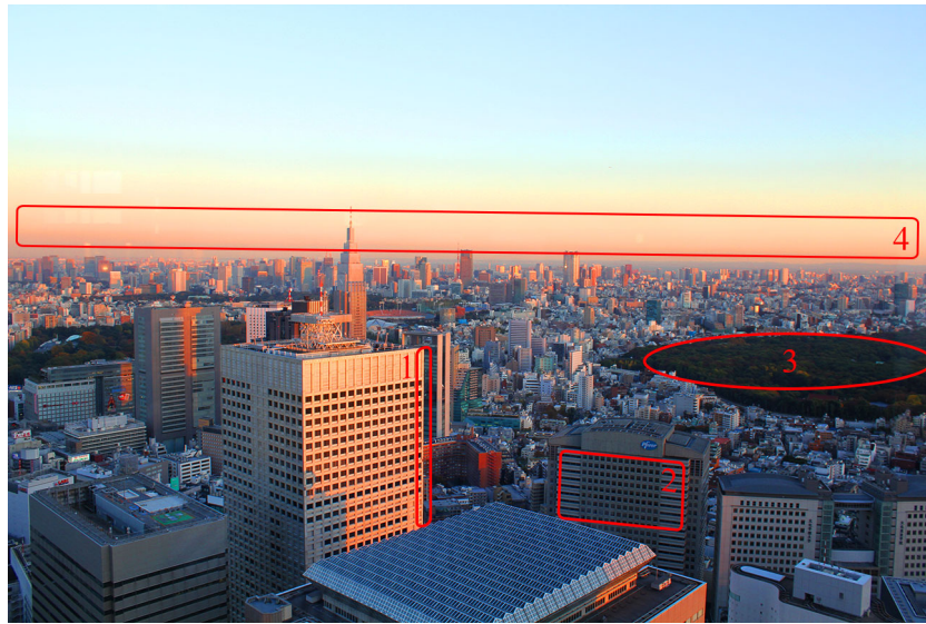
Figure 1.1: All marked areas show different edge types. 1. contour or structural edge, 2. edges on a planar surface, 3. edges as a result of a mixture of complex texture and three-dimensional structure, 4. soft edges that describe a smooth brightness or even color transition.
