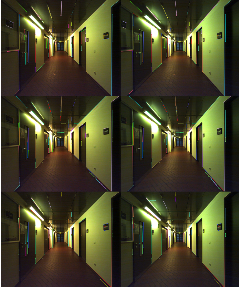
Figure 3.19: Exemplary line match result for the Corridor sequence. Matching line segments have corresponding colors in the left and right image. Top row: line matching, middle row: EBDP, bottom row: EMCBR.
