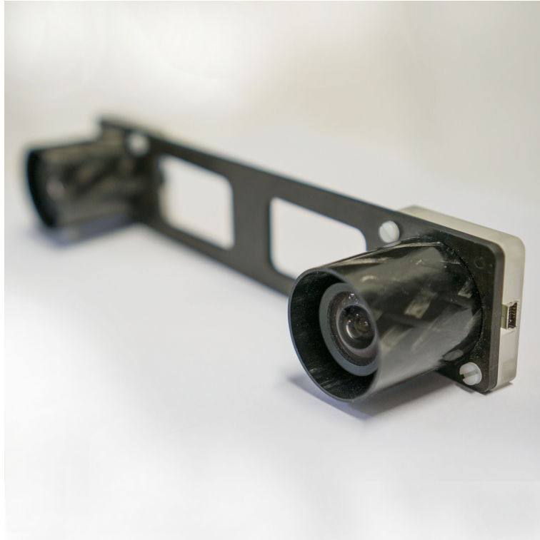
Figure 2.4: The custom stereo camera that was used for the acquisition of all sequences in this thesis. The baseline is 16cm and the field-of-view is 100^\circ \times 80^\circ .
