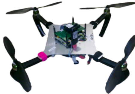
Figure A.1: The iQCopter quadrotor MAV. The highest point is the IMU to achieve the largest possible separation between the actuator currents and the magnetometers. The iQCopter measures 72cm from rotor tip to rotor tip and weighs about 1250 grams including a 3300mAh 3-cell lithium polymer battery.
