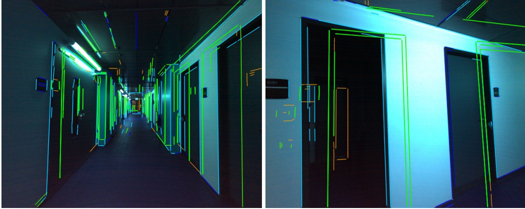
Figure 4.6: These images show initial matching configurations of the Corridor sequence. ICML was able to register the lines without sample consensus matching. ICP falls into local minima on the shown setups, because some of the closest lines are false matches. The images show the initial reprojection of the previous frame prior to registration with d_{\max} = d_{\text{init}} = 64\text{px} . Green depicts matched reprojected model lines, while unmatched ones are drawn in orange. Detected image lines are cyan if they were matched and dark blue for non-matched ones.
